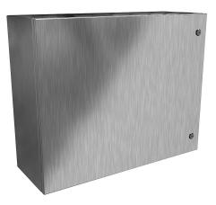
Hammond Eclipse series enclosure, NEMA 3R/4/4X/12/13,  $24 \times 30 \times 10$  in (HxWxD), wall mount, 304 stainless steel, #4 brush finish, single-door, 1/4-turn semi-flush 316 stainless steel latch.
