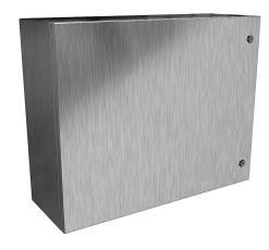
Hammond Eclipse series enclosure, NEMA 3R/4/4X/12/13,  $24 \times 30 \times 10$  in (HxWxD), wall mount, 316 stainless steel, #4 brush finish, single-door, 1/4-turn semi-flush 316 stainless steel latch.
