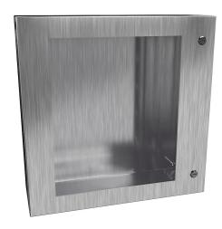
Hammond Eclipse series enclosure, NEMA 3R/4/4X/12/13,  $24 \times 24 \times 8$  in (HxWxD), wall mount, 304 stainless steel, #4 brush finish, single-door, 1/4-turn semi-flush 316 stainless steel latch, polycarbonate window.
