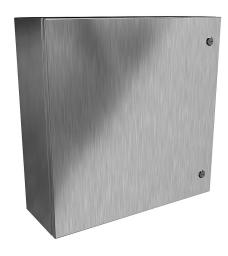
Hammond Eclipse series enclosure, NEMA 3R/4/4X/12/13, 24 x 24 x 8in (HxWxD), wall mount, 304 stainless steel, #4 brush finish, single-door, 1/4-turn semi-flush 316 stainless steel latch.
