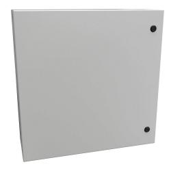
Hammond Eclipse series enclosure, NEMA 3R/4/12,  $24 \times 24 \times 8in$  (HxWxD), wall mount, carbon steel, RAL 7035 light gray, powder coat finish, single-door, 1/4-turn semi-flush latch.
