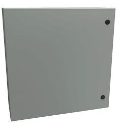
Hammond Eclipse series enclosure, NEMA 3R/4/12, 24 x 24 x 8in (HxWxD), wall mount, carbon steel, ANSI 61 gray, powder coat finish, single-door, 1/4-turn semi-flush latch.
