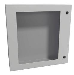
Hammond Eclipse series enclosure, NEMA 3R/4/12,  $24 \times 24 \times 6in$  (HxWxD), wall mount, carbon steel, RAL 7035 light gray, powder coat finish, single-door, 1/4-turn semi-flush latch, polycarbonate window.
