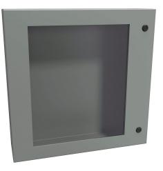
Hammond Eclipse series enclosure, NEMA 3R/4/12, 24 x 24 x 6in (HxWxD), wall mount, carbon steel, ANSI 61 gray, powder coat finish, single-door, 1/4-turn semi-flush latch, polycarbonate window.
