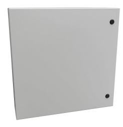
Hammond Eclipse series enclosure, NEMA 3R/4/12, 24 x 24 x 6in (HxWxD), wall mount, carbon steel, RAL 7035 light gray, powder coat finish, single-door, 1/4-turn semi-flush latch.
