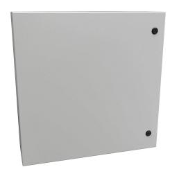
Hammond Eclipse series enclosure, NEMA 3R/4/12,  $24 \times 24 \times 6in$  (HxWxD), wall mount, carbon steel, RAL 7035 light gray, powder coat finish, single-door, 1/4-turn semi-flush latch.
