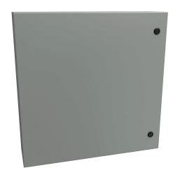
Hammond Eclipse series enclosure, NEMA 3R/4/12,  $24 \times 24 \times 6in$  (HxWxD), wall mount, carbon steel, ANSI 61 gray, powder coat finish, single-door, 1/4-turn semi-flush latch.
