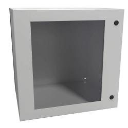
Hammond Eclipse series enclosure, NEMA 3R/4/12, 24 x 24 x 20in (HxWxD), wall mount, carbon steel, RAL 7035 light gray, powder coat finish, single-door, 1/4-turn semi-flush latch, polycarbonate window.
