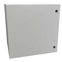
Hammond Eclipse series enclosure, NEMA 3R/4/12, 24 x 24 x 20in (HxWxD), wall mount, carbon steel, RAL 7035 light gray, powder coat finish, single-door, 1/4-turn semi-flush latch.
