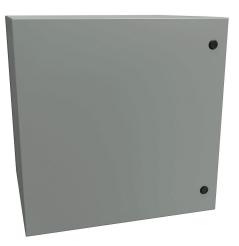
Hammond Eclipse series enclosure, NEMA 3R/4/12, 24 x 24 x 20in (HxWxD), wall mount, carbon steel, ANSI 61 gray, powder coat finish, single-door, 1/4-turn semi-flush latch.
