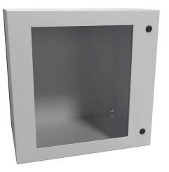
Hammond Eclipse series enclosure, NEMA 3R/4/12, 24 x 24 x 16in (HxWxD), wall mount, carbon steel, RAL 7035 light gray, powder coat finish, single-door, 1/4-turn semi-flush latch, polycarbonate window.
