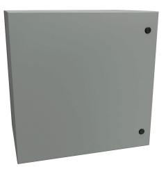
Hammond Eclipse series enclosure, NEMA 3R/4/12, 24 x 24 x 16in (HxWxD), wall mount, carbon steel, ANSI 61 gray, powder coat finish, single-door, 1/4-turn semi-flush latch.
