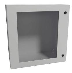
Hammond Eclipse series enclosure, NEMA 3R/4/12, 24 x 24 x 12in (HxWxD), wall mount, carbon steel, RAL 7035 light gray, powder coat finish, single-door, 1/4-turn semi-flush latch, polycarbonate window.
