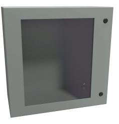
Hammond Eclipse series enclosure, NEMA 3R/4/12, 24 x 24 x 12in (HxWxD), wall mount, carbon steel, ANSI 61 gray, powder coat finish, single-door, 1/4-turn semi-flush latch, polycarbonate window.
