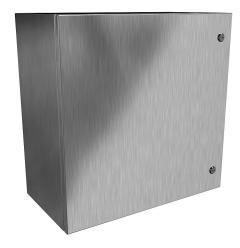
Hammond Eclipse series enclosure, NEMA 3R/4/4X/12/13,  $24 \times 24 \times 12$  in (HxWxD), wall mount, 304 stainless steel, #4 brush finish, single-door, 1/4-turn semi-flush 316 stainless steel latch.
