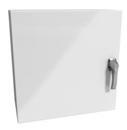
Hammond Eclipse series enclosure, NEMA 3R/4/4X/12/13,  $24 \times 24 \times 12$  in (HxWxD), wall mount, 304 stainless steel, RAL 9003 white, powder coat finish, single-door, 3-point 316 stainless steel padlocking handle.
