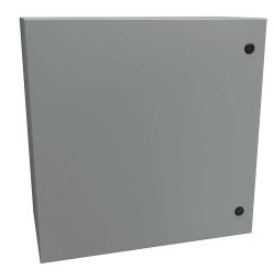
Hammond Eclipse series enclosure, NEMA 3R/4/12, 24 x 24 x 12in (HxWxD), wall mount, carbon steel, ANSI 61 gray, powder coat finish, single-door, 1/4-turn semi-flush latch.
