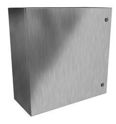
Hammond Eclipse series enclosure, NEMA 3R/4/4X/12/13,  $24 \times 24 \times 10$  in (HxWxD), wall mount, 304 stainless steel, #4 brush finish, single-door, 1/4-turn semi-flush 316 stainless steel latch.
