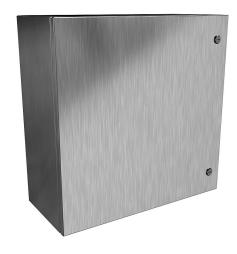
Hammond Eclipse series enclosure, NEMA 3R/4/4X/12/13,  $24 \times 24 \times 10$  in (HxWxD), wall mount, 316 stainless steel, #4 brush finish, single-door, 1/4-turn semi-flush 316 stainless steel latch.
