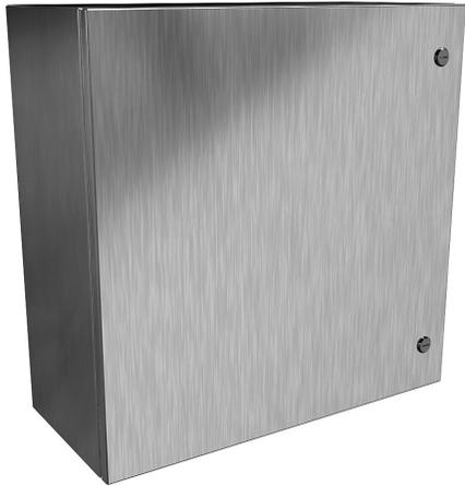
Hammond Eclipse series enclosure, NEMA 3R/4/4X/12/13, 24 x 24 x 10in (HxWxD), wall mount, 316 stainless steel, #4 brush finish, single-door, 1/4-turn semi-flush 316 stainless steel latch.
