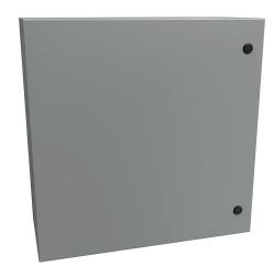
Hammond Eclipse series enclosure, NEMA 3R/4/12, 24 x 24 x 10in (HxWxD), wall mount, carbon steel, ANSI 61 gray, powder coat finish, single-door, 1/4-turn semi-flush latch.
