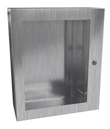
Hammond Eclipse series enclosure, NEMA 3R/4/4X/12/13,  $24 \times 20 \times 8$  in (HxWxD), wall mount, 304 stainless steel, #4 brush finish, single-door, 1/4-turn semi-flush 316 stainless steel latch, polycarbonate window.
