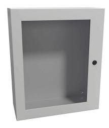
Hammond Eclipse series enclosure, NEMA 3R/4/12, 24 x 20 x 8in (HxWxD), wall mount, carbon steel, RAL 7035 light gray, powder coat finish, single-door, 1/4-turn semi-flush latch, polycarbonate window.
