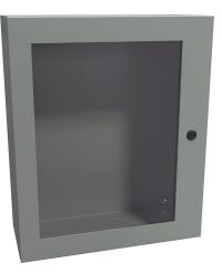
Hammond Eclipse series enclosure, NEMA 3R/4/12, 24 x 20 x 8in (HxWxD), wall mount, carbon steel, ANSI 61 gray, powder coat finish, single-door, 1/4-turn semi-flush latch, polycarbonate window.
