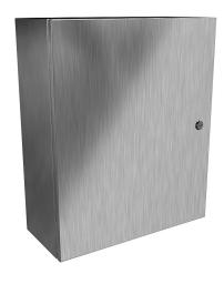
Hammond Eclipse series enclosure, NEMA 3R/4/4X/12/13, 24 x 20 x 8in (HxWxD), wall mount, 304 stainless steel, #4 brush finish, single-door, 1/4-turn semi-flush 316 stainless steel latch.
