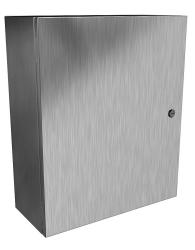
Hammond Eclipse series enclosure, NEMA 3R/4/4X/12/13, 24 x 20 x 8in (HxWxD), wall mount, 316 stainless steel, #4 brush finish, single-door, 1/4-turn semi-flush 316 stainless steel latch.
