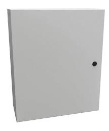
Hammond Eclipse series enclosure, NEMA 3R/4/12,  $24 \times 20 \times 8in$  (HxWxD), wall mount, carbon steel, RAL 7035 light gray, powder coat finish, single-door, 1/4-turn semi-flush latch.
