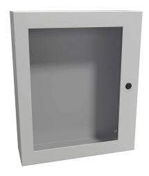
Hammond Eclipse series enclosure, NEMA 3R/4/12,  $24 \times 20 \times 6$ in (HxWxD), wall mount, carbon steel, RAL 7035 light gray, powder coat finish, single-door, 1/4-turn semi-flush latch, polycarbonate window.
