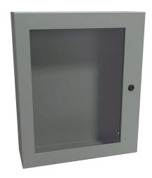
Hammond Eclipse series enclosure, NEMA 3R/4/12, 24 x 20 x 6in (HxWxD), wall mount, carbon steel, ANSI 61 gray, powder coat finish, single-door, 1/4-turn semi-flush latch, polycarbonate window.
