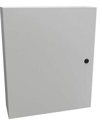
Hammond Eclipse series enclosure, NEMA 3R/4/12, 24 x 20 x 6in (HxWxD), wall mount, carbon steel, RAL 7035 light gray, powder coat finish, single-door, 1/4-turn semi-flush latch.
