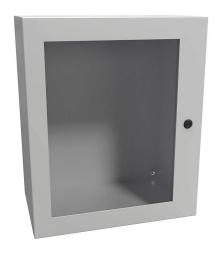
Hammond Eclipse series enclosure, NEMA 3R/4/12, 24 x 20 x 12in (HxWxD), wall mount, carbon steel, RAL 7035 light gray, powder coat finish, single-door, 1/4-turn semi-flush latch, polycarbonate window.
