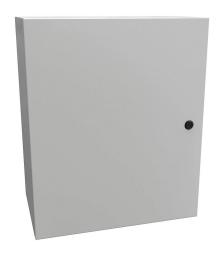
Hammond Eclipse series enclosure, NEMA 3R/4/12,  $24 \times 20 \times 12$ in (HxWxD), wall mount, carbon steel, RAL 7035 light gray, powder coat finish, single-door, 1/4-turn semi-flush latch.
