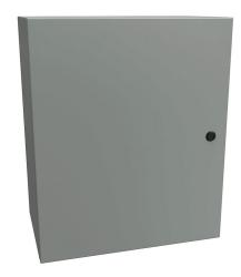
Hammond Eclipse series enclosure, NEMA 3R/4/12, 24 x 20 x 12in (HxWxD), wall mount, carbon steel, ANSI 61 gray, powder coat finish, single-door, 1/4-turn semi-flush latch.
