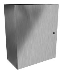
Hammond Eclipse series enclosure, NEMA 3R/4/4X/12/13,  $24 \times 20 \times 10$  in (HxWxD), wall mount, 304 stainless steel, #4 brush finish, single-door, 1/4-turn semi-flush 316 stainless steel latch.
