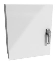
Hammond Eclipse series enclosure, NEMA 3R/4/4X/12/13,  $24 \times 20 \times 10$  in (HxWxD), wall mount, 304 stainless steel, RAL 9003 white, powder coat finish, single-door, 3-point 316 stainless steel padlocking handle.
