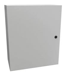
Hammond Eclipse series enclosure, NEMA 3R/4/12,  $24 \times 20 \times 10$ in (HxWxD), wall mount, carbon steel, RAL 7035 light gray, powder coat finish, single-door, 1/4-turn semi-flush latch.
