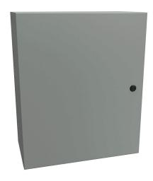
Hammond Eclipse series enclosure, NEMA 3R/4/12, 24 x 20 x 10in (HxWxD), wall mount, carbon steel, ANSI 61 gray, powder coat finish, single-door, 1/4-turn semi-flush latch.
