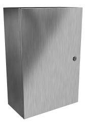
Hammond Eclipse series enclosure, NEMA 3R/4/4X/12/13, 24 x 16 x 8in (HxWxD), wall mount, 304 stainless steel, #4 brush finish, single-door, 1/4-turn semi-flush 316 stainless steel latch.
