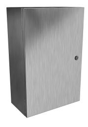
Hammond Eclipse series enclosure, NEMA 3R/4/4X/12/13, 24 x 16 x 8in (HxWxD), wall mount, 316 stainless steel, #4 brush finish, single-door, 1/4-turn semi-flush 316 stainless steel latch.
