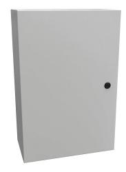
Hammond Eclipse series enclosure, NEMA 3R/4/12,  $24 \times 16 \times 8in$  (HxWxD), wall mount, carbon steel, RAL 7035 light gray, powder coat finish, single-door, 1/4-turn semi-flush latch.
