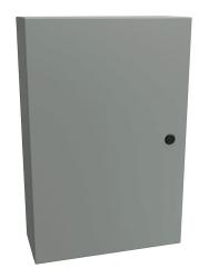
Hammond Eclipse series enclosure, NEMA 3R/4/12,  $24 \times 16 \times 6$ in (HxWxD), wall mount, carbon steel, ANSI 61 gray, powder coat finish, single-door, 1/4-turn semi-flush latch.
