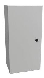
Hammond Eclipse series enclosure, NEMA 3R/4/12,  $24 \times 12 \times 8in$  (HxWxD), wall mount, carbon steel, RAL 7035 light gray, powder coat finish, single-door, 1/4-turn semi-flush latch.
