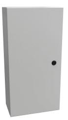
Hammond Eclipse series enclosure, NEMA 3R/4/12,  $24 \times 12 \times 6in$  (HxWxD), wall mount, carbon steel, RAL 7035 light gray, powder coat finish, single-door, 1/4-turn semi-flush latch.
