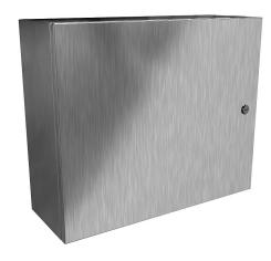
Hammond Eclipse series enclosure, NEMA 3R/4/4X/12/13,  $20 \times 24 \times 8$  in (HxWxD), wall mount, 304 stainless steel, #4 brush finish, single-door, 1/4-turn semi-flush 316 stainless steel latch.
