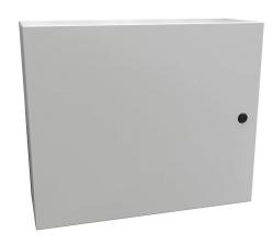
Hammond Eclipse series enclosure, NEMA 3R/4/12,  $20 \times 24 \times 8in$  (HxWxD), wall mount, carbon steel, RAL 7035 light gray, powder coat finish, single-door, 1/4-turn semi-flush latch.
