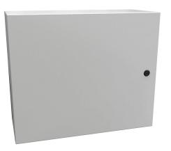
Hammond Eclipse series enclosure, NEMA 3R/4/12, 20 x 24 x 10in (HxWxD), wall mount, carbon steel, RAL 7035 light gray, powder coat finish, single-door, 1/4-turn semi-flush latch.
