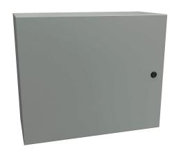
Hammond Eclipse series enclosure, NEMA 3R/4/12,  $20 \times 24 \times 10$ in (HxWxD), wall mount, carbon steel, ANSI 61 gray, powder coat finish, single-door, 1/4-turn semi-flush latch.
