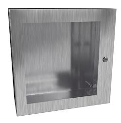
Hammond Eclipse series enclosure, NEMA 3R/4/4X/12/13,  $20 \times 20 \times 8$  in (HxWxD), wall mount, 304 stainless steel, #4 brush finish, single-door, 1/4-turn semi-flush 316 stainless steel latch, polycarbonate window.
